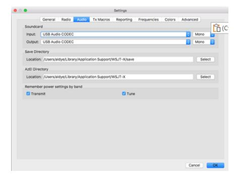
Move to the Audio Tab. Select USB Audio Codec on both input and output.
